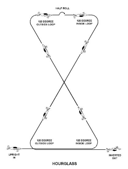
From level flight perform a 1/3 inside loop through approximately 120 degrees to inverted 60 degree climb. At the top of the climb perform a 1/3 outside loop to level flight. Half roll to inverted. Perform a 1/3 inside loop through approximately 120 degrees to upright 60 degree dive. Perform a 1/3 outside loop through approximately 120 degrees to level flight, exit inverted.
