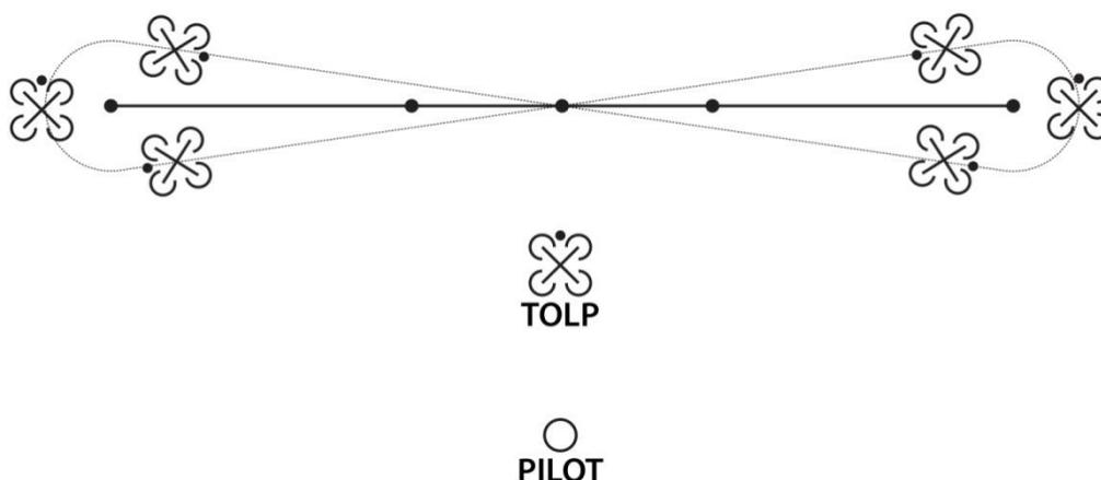
**At no time during the manoeuvre should the model be flying sideways. Throughout all the turns and straight flight, it must be flying forward in the hover and not ‘crabbing’ sideways.**
