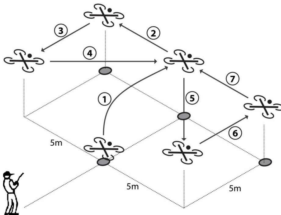
(1) The model starts on the TOLP, takes off and flies to a position over the centre marker where it is hovered for about 5 seconds.
