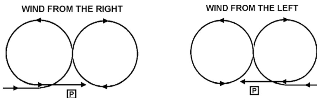
This should be flown as a banked circuit manoeuvre (not from the hover) and as shown in the diagram. The crossover point must always be in front of the pilot and, after a run in at standard height and line, the model MUST be turned through ninety degrees in the first turn so that it is flying exactly away from the pilot.
